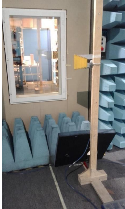
Figure 49: Receiving antenna moving vertically from point B
