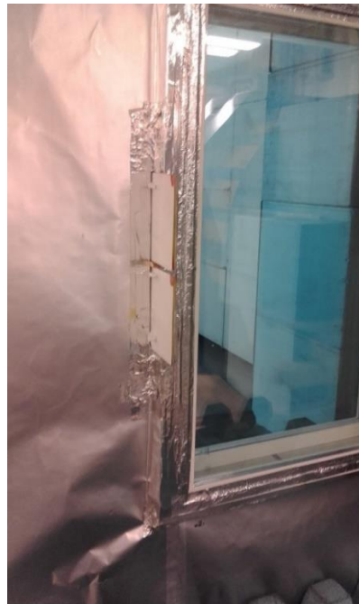
Figure 69: Two passive repeaters in the center
