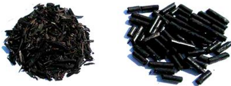
Figure 1. Torrefied biomass a.k.a. “bio coal”, before and after densification process. (conBio 2013)
