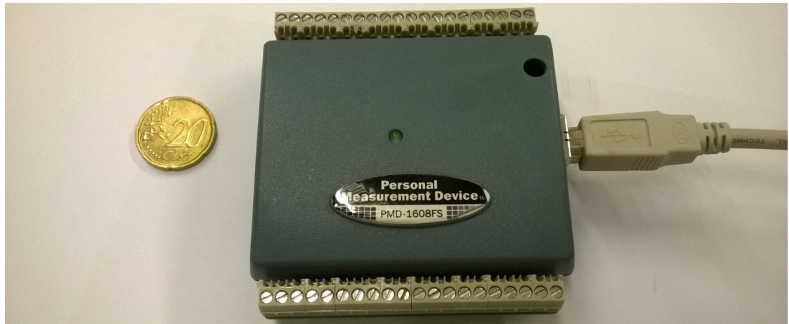
Figure 23. USB data acquisition system from Measurement Computing.
