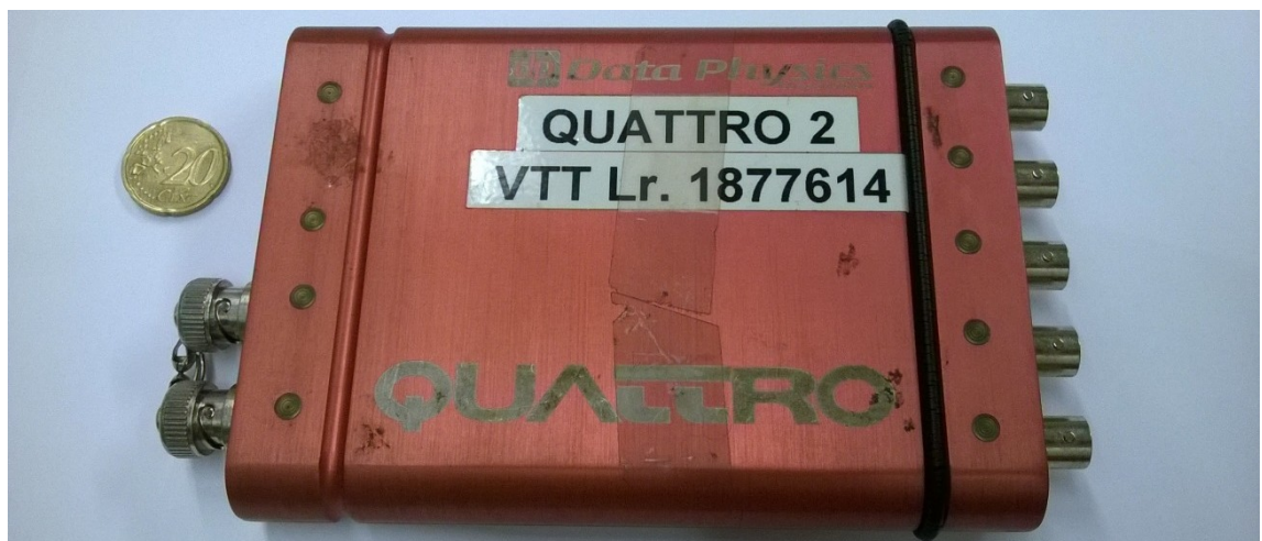
Figure 24. USB DAQ from Data Physics made for industrial measurements.
