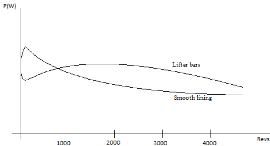
Figure 10. An illustration of net power alteration during grindability test. Modified from the source. (Niitti, 1970)
