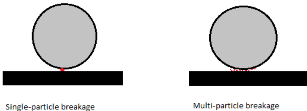
Figure 3. Illustration of single-particle and multi-particle breakage event. Modified from the source. (Fuerstenau & Han, 2003)
