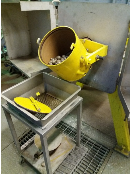
Figure 26. The Mergan mill used in tests, positioned for filling
