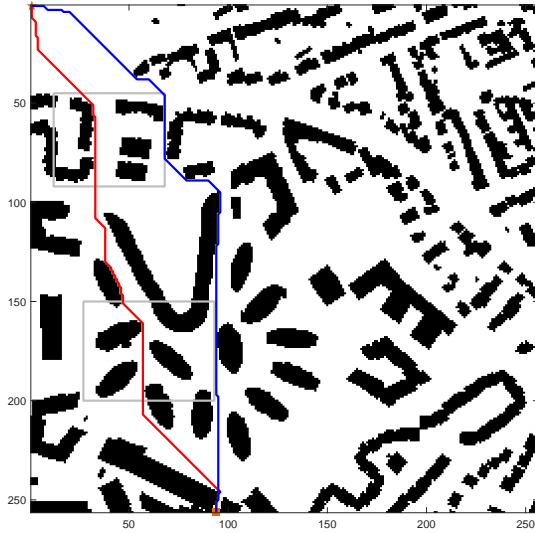
(a) Shortest path calculation for robotic path planning
