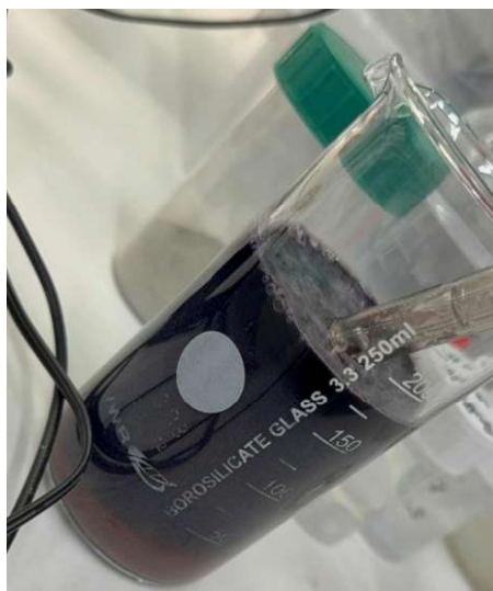
Figure 4. A sample after mixing milled phlogopite with acids ( H_2SO_4 & DHZ).
