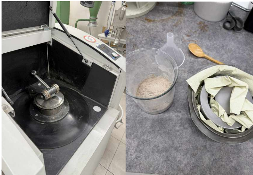
Figure 3. The disk mill RS200 used for milling phlogopite.
