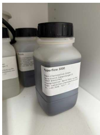
Figure 2. A polycarboxylate-based superplasticizer (Hyperflow 3000, Rhein-Chemotechnik GmbH, Germany)
