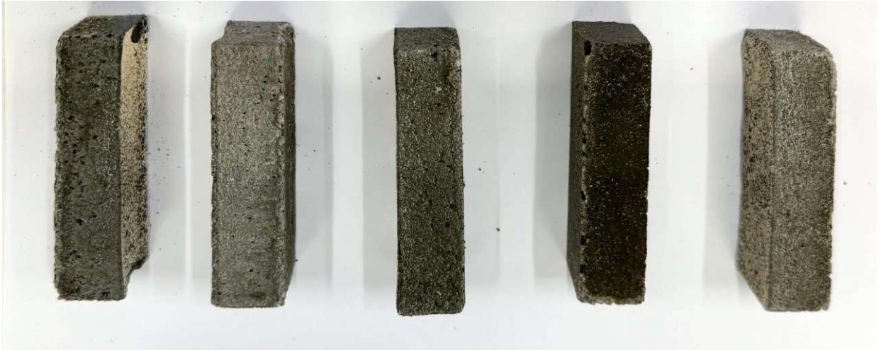
Figure 10. All samples after curing arranged from left to right: Ref-Cement, Raw-Phlog-Cement, Mill-Phlog-Cement, H_2SO_4 -Cement and DHZ-Cement.
