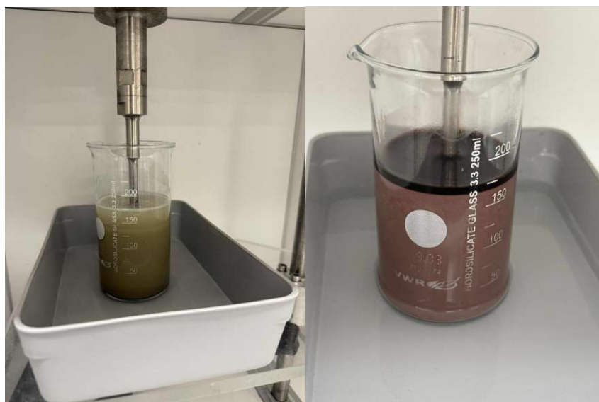
Figure 5. The picture on the left was the leaching process of the phlogopite sample using 0.1M of sulfuric acid ( H_2SO_4 ) and picture on the right was the leaching process of the phlogopite sample using 0.1M of DHZ and 0.1M of sulfuric acid ( H_2SO_4 ).
