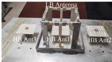
Fig. 13. A bow-shaped LB antenna with an embedded HB antenna in it [92].
