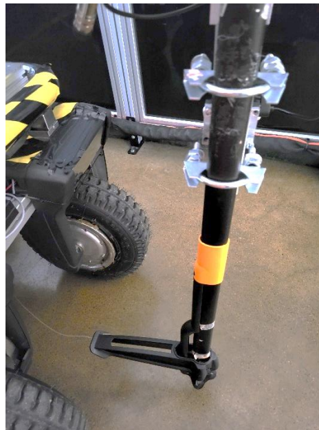
Figure 12. Fiskars Xact weed puller attached to the robot.
