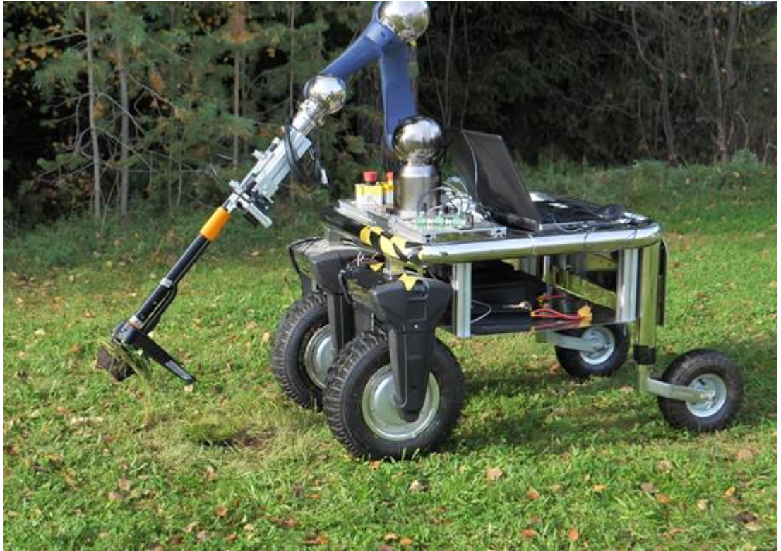
Figure 34. Pulling the weed from the ground with the weeding tool.
