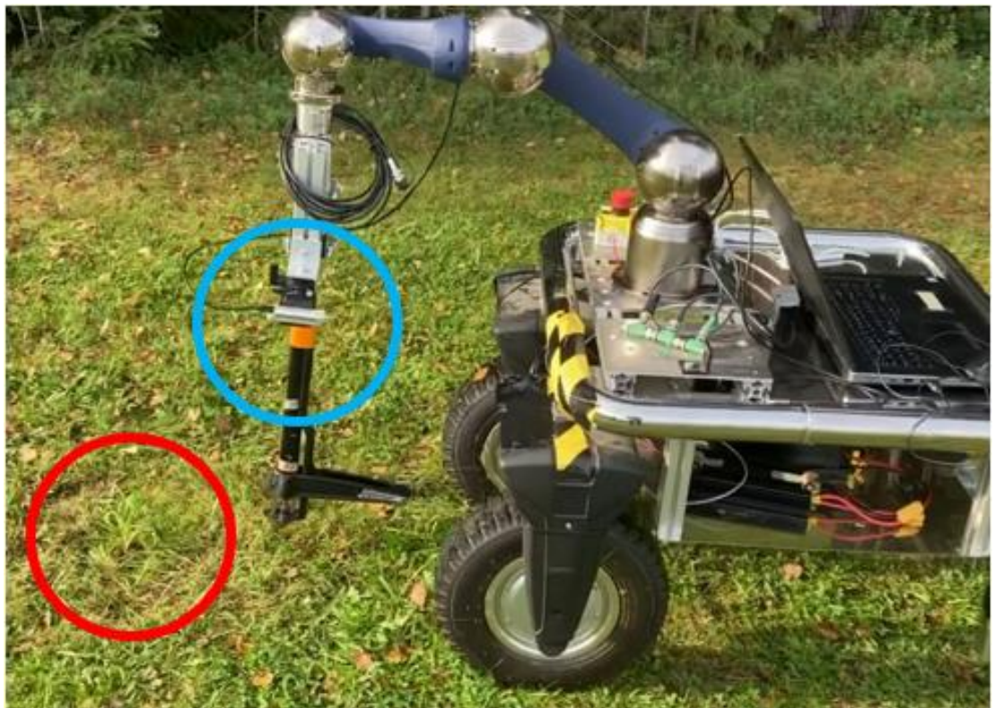
Figure 32. Detecting the weed on the ground. Red is the weed and blue is the camera.
