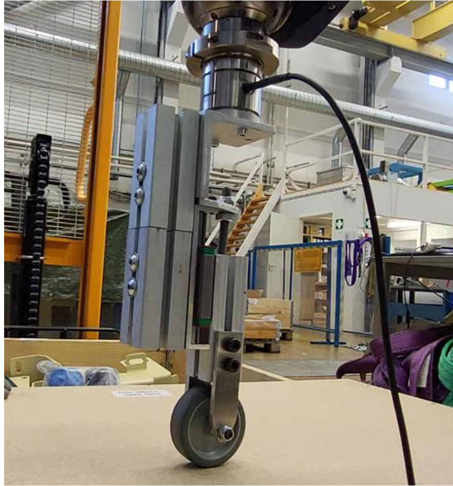
Figure 29. Force control test with a spring-loaded track and a wheel attached to the robot flange.
