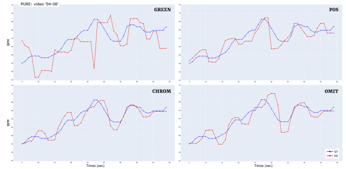
Fig. 9. Comparison of HR estimation using four rPPG methods with the Multi-region pipeline. Estimated heart rate (red) is extracted from the face, and the contact-based reference PPG signal (blue) is computed on a single PURE dataset video.
