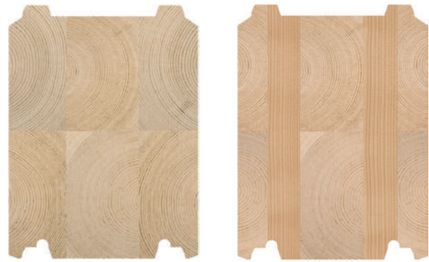
Fig. 6. Cross-sections (275mm x 205mm) of a traditional, settling lamella log (left) and a non-settling log. Logs become “non-settling”, when they are glued together from crossing lamellas, since inside the log, there is vertical wood, which nearly eliminates the shrinkage of the log in a vertical direction. Image: Kontio Log Houses. (Published with permission)
