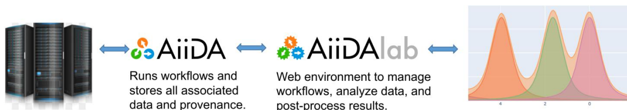
Figure 1: Run XPS calculations using AiiDA workflow via tailored lightweight AiiDALab web applications directly in the browser.
