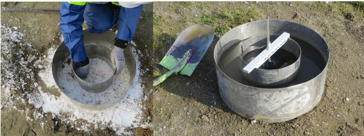
Figure 24. Double-ring infiltrometer, mostly used for the in situ hydraulic conductivity test method (Anne Tuomela)
