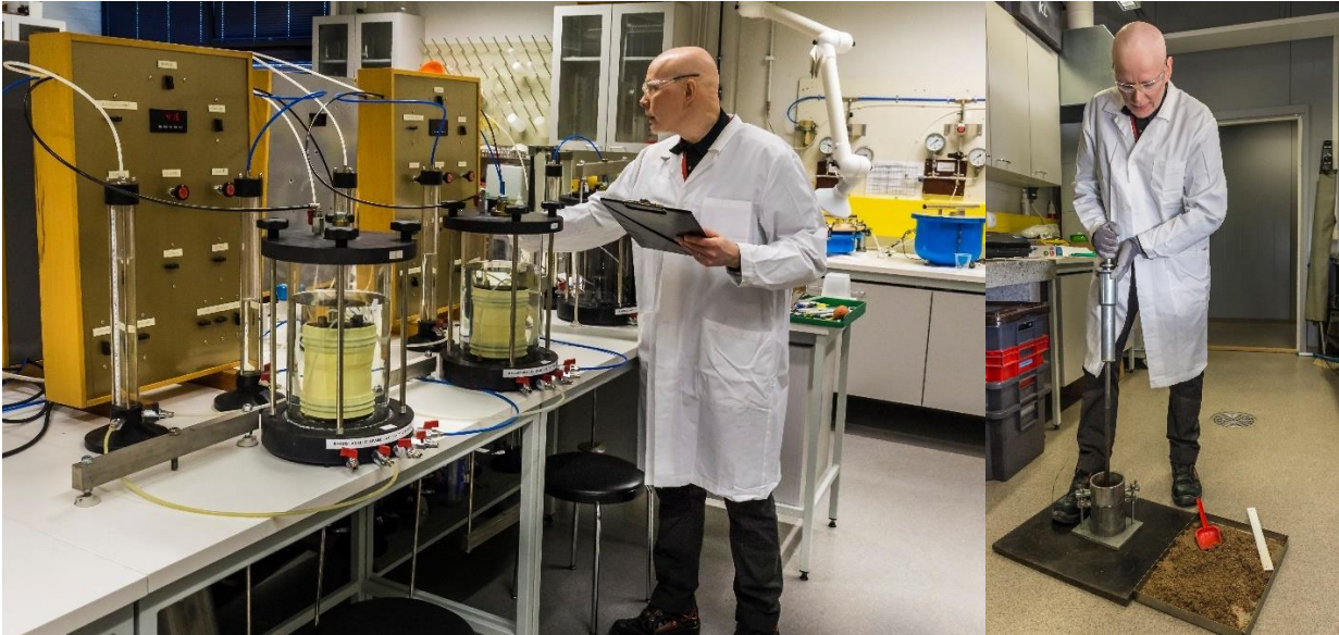
Figure 23. Left: Hydraulic conductivity or permeability can be measured using several methods in the laboratory. The figure shows flexible-wall permeability cells. Right: The Proctor experiment can be used to find out the parameters associated with the compaction of the material.
