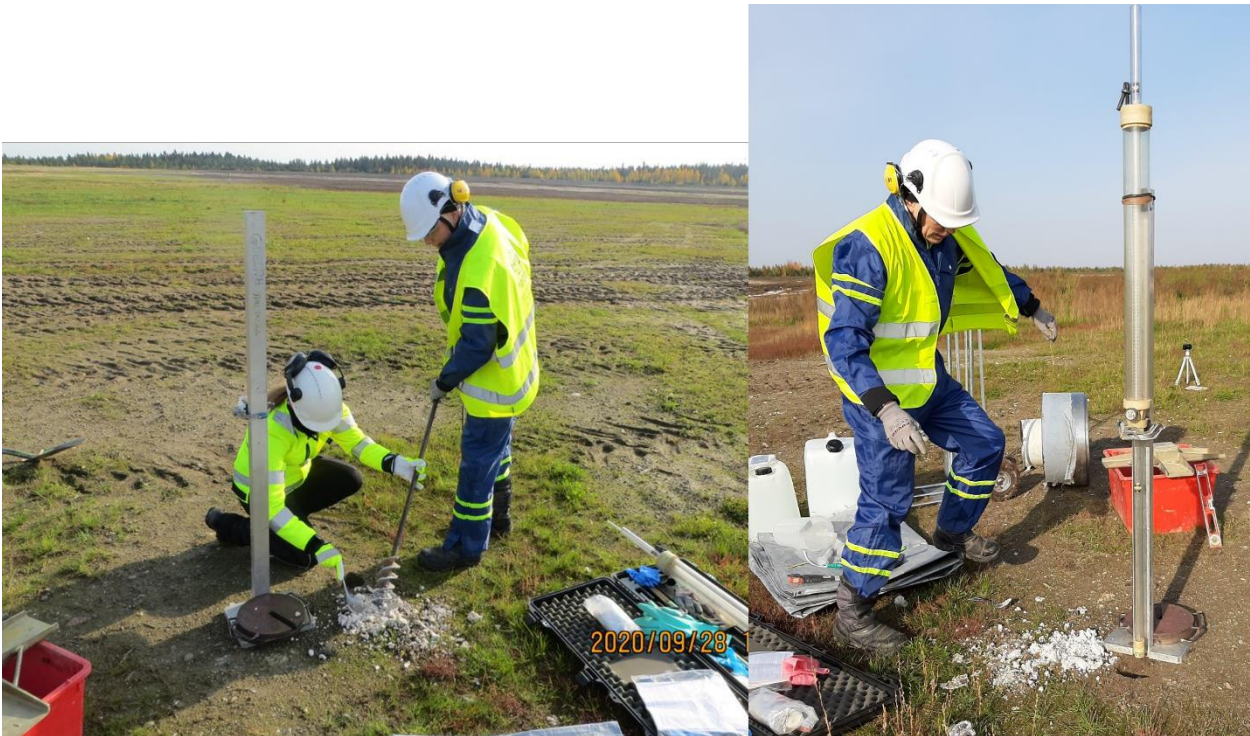
Figure 25. The Guelph infiltrometer can measure a lower hydraulic conductivity level (compared with the double-ring infiltrometer) and can be used in deeper soil (Anne Tuomela)
