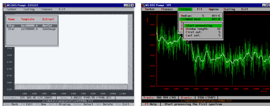
Figure A.1: Left : An image with the selected overscan area in the CCD columns shown as the marker box. The position of the box is given in the highlighted record of the opened list of regions. Right : An averaged bias column containing a jump in it due to CCD electronics stabilization problem is shown. A trimmed mean filter is used to eliminate the readout noise and preserve the variations. The smoothed bias is subtracted from every column of the original image.
