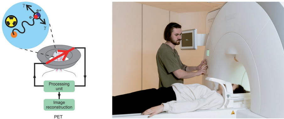
Figure 1. The principle of PET scanning simplified from Ref. [6]. The emitted positron collides with an electron, then annihilation will happen. The basis of this phenomenon is the emission of two same-energy gamma photons in opposite directions. Finally, gamma detectors capture the photons and process them to reconstruct a 3D image. On the right, preparations to start brain imaging (Photo by MART PRODUCTION from pexels.com).
