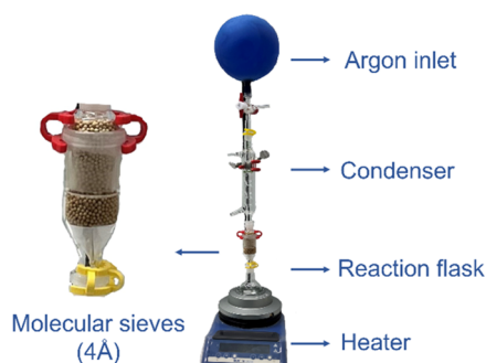
Figure 2. Designed polycondensation system under atmospheric pressure.
