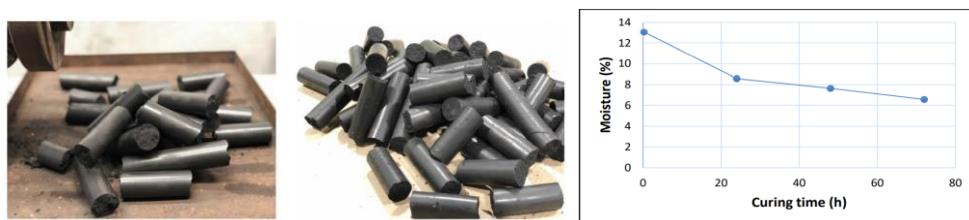
Figure 2. Left: Kivisampo briquettes pictured before and after the curing step. Right: The dependence of moisture content on time after molding.
