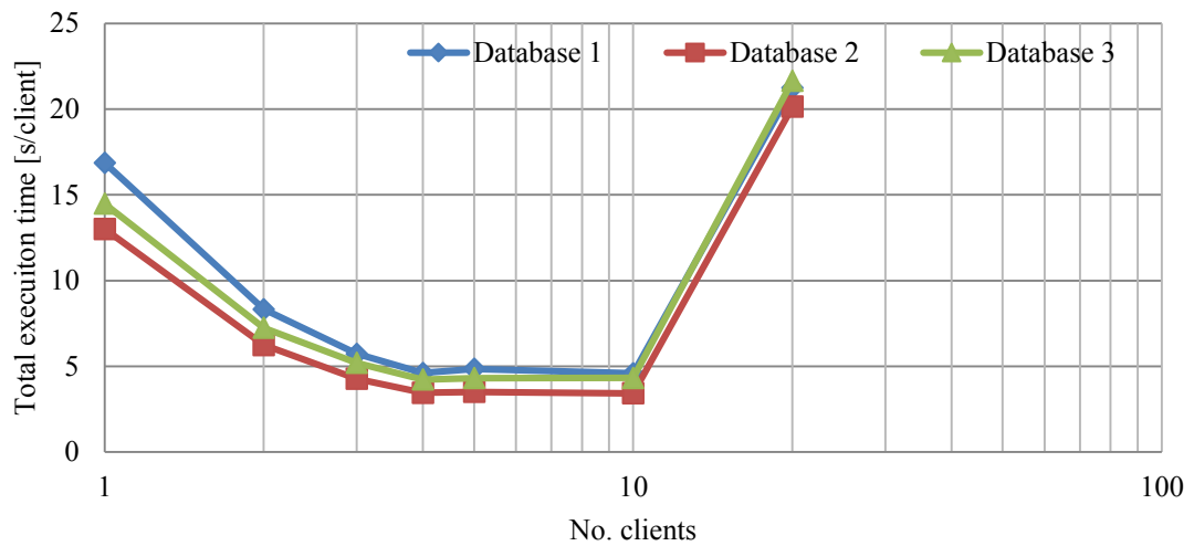
Figure 5.12. Total execution time against the number of clients for Case 4 in Query 1.
