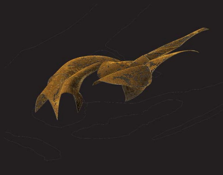
Below: Axonometric projection of the perforated canopy construction. The colours correspond with the colours of the picture on the previous page; they have been mapped to varying sized openings.
