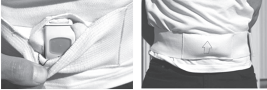
Fig. 2. Wireless sensor for acceleration measurements in real life worn on the waist with an elastic belt. The vertical axis of the system was marked as an arrow on the belt.
