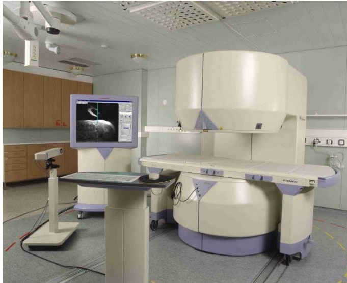
Fig. 1. An open interventional MRI system.
