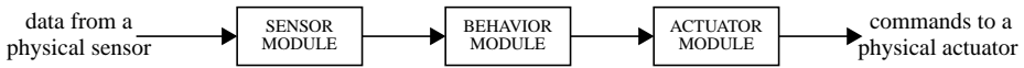
Fig. 3. A basic signal path of a behavior-based system. This path from perception to action is specialized into achieving a simple goal.
