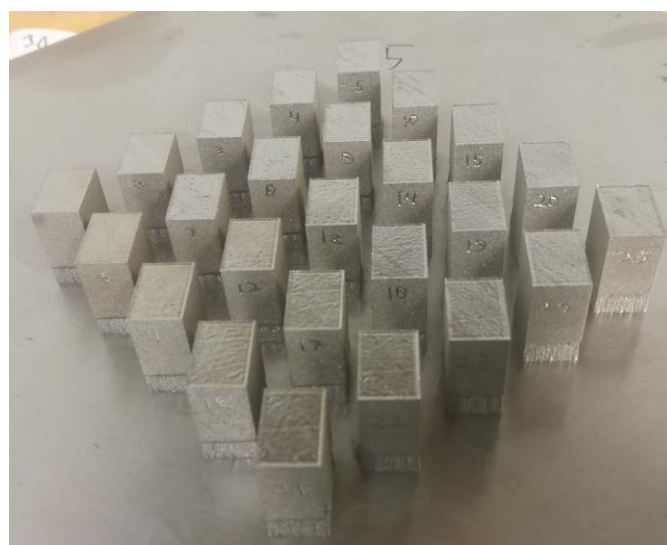
Fig. 2. The platform of cubes printed with the varied parameters for the edges.
