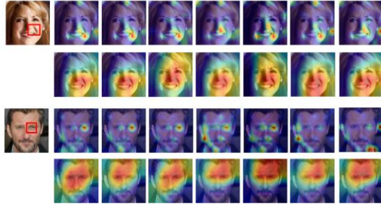
Fig. 6. Classification activation maps of the shallow layer and deep layer under different post-processing operations. For each image, the first row is for the shallow layer, while the second row is for the deep layer. For each row, from left to right, images correspond to the original image and its maps, the maps of JPEG compression, Gaussian noise, Gaussian blurring, gamma correction, median filtering and resizing.
