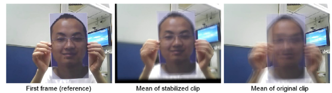
Fig. 2. First frame of a sample print attack video clip (left) and the mean of the corresponding stabilized video clip (middle). The result of simple frame averaging (right) is included for comparison to demonstrate the amount of inter-frame 2D affine motion in the original print attack video clip.
