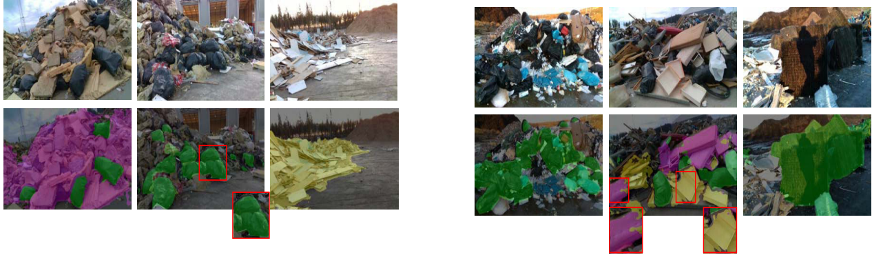
Fig. 5. Semantic segmentation results for material recycling Row 1: Original Image, Row 2: Test set segmented results. Indicated red box regions in which we perform better in some classes(Plastic, Wood, Sponge)
