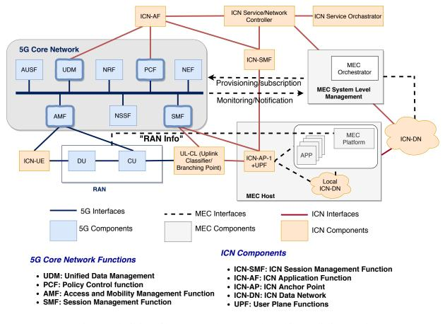
Fig. 3: A depiction of how ICN and MEC can be architecturally integrated.
