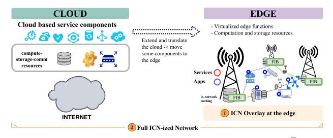
Fig. 1: Integration of ICN and MEC in 5G. ICN is a beneficial enabler for the edge computing scenarios (1) while it can be a much more fundamental networking technology in the long run (2).
