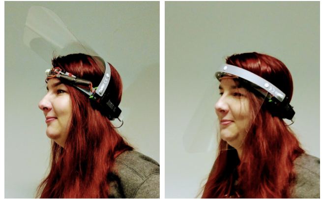
Figure 2: The dynamic face visor in open and closed positions. An additional LED to indicate when a coughing sound has been recognized is included for development purposes.
