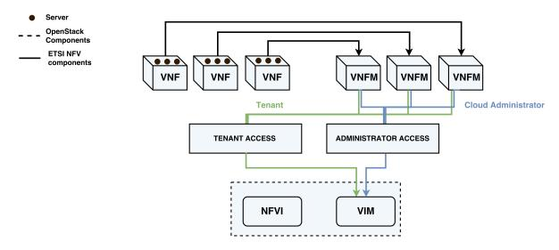
Fig. 3: Example of mapping of VNFs and VMs on an OpenStack IaaS.
