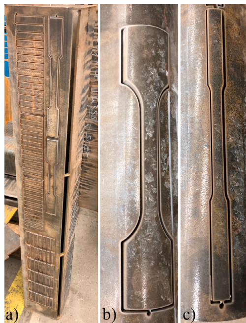
Fig. 2. Examples of water-cutted Charpy-V impact toughness and tensile test samples from (a) flat side and (b-c) corner of rectangular hollow section. Two types of tensile test ((b) wide and (c) narrow) specimen from corner were used.
