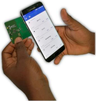
Figure 7. Demonstration of how data is collected using the S3 application and the SensorCard.
