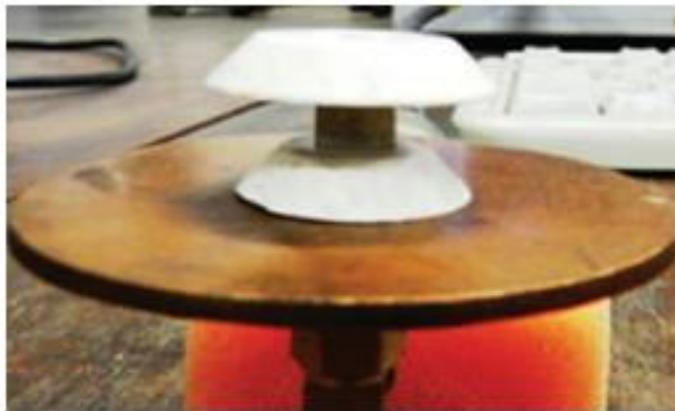
FIGURE 7. The fabricated mushroom-shaped DRA with h_1 = 4.2 , h_2 = 5.1 , h_3 = 4.2 , LDR1 = 17.6 , LDR2 = 6 , LDR3 = 22.2 , b = 1.57 , fr_1 = 6.5 , fr_2 = 4.5 , fr_2 = 4 , and l = 11 . (All dimensions are in millimeters.)
