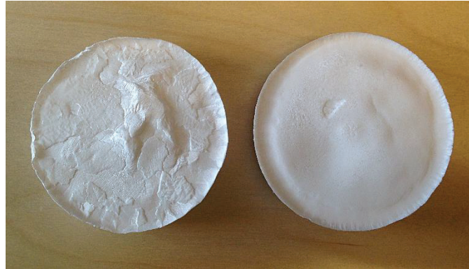
FIGURE 2. Appearance of PVA foams with CNCs prepared by keeping the solution at -20\text{ }^{\circ}\text{C} for 48 h (left) and using liquid nitrogen (right).
