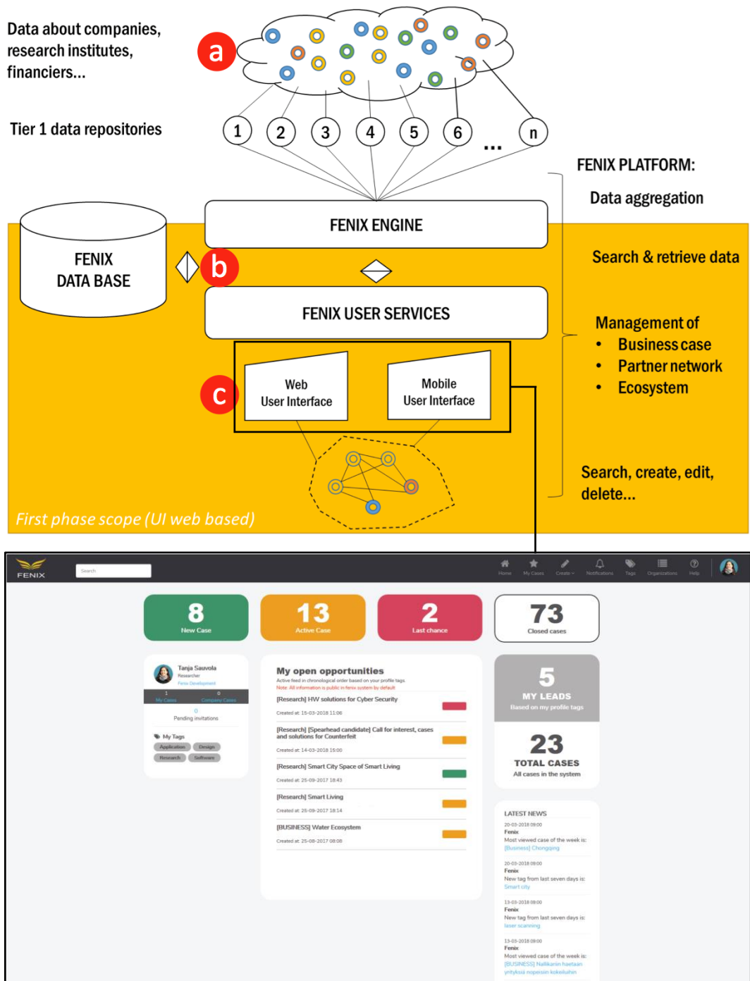
Figure 3. Fenix implementation and UI. (a) Organizations fill in their data on Fenix system and select suitable tags to present their organizations interests and expertise. Similarly, cases are initiated based on the description and tags. (b) Fenix system compares the tags and creates a list of potential partners if the distance between the tags is below a certain threshold. (c) A list of potential partners is then presented to users with a possibility to send an invitation.
