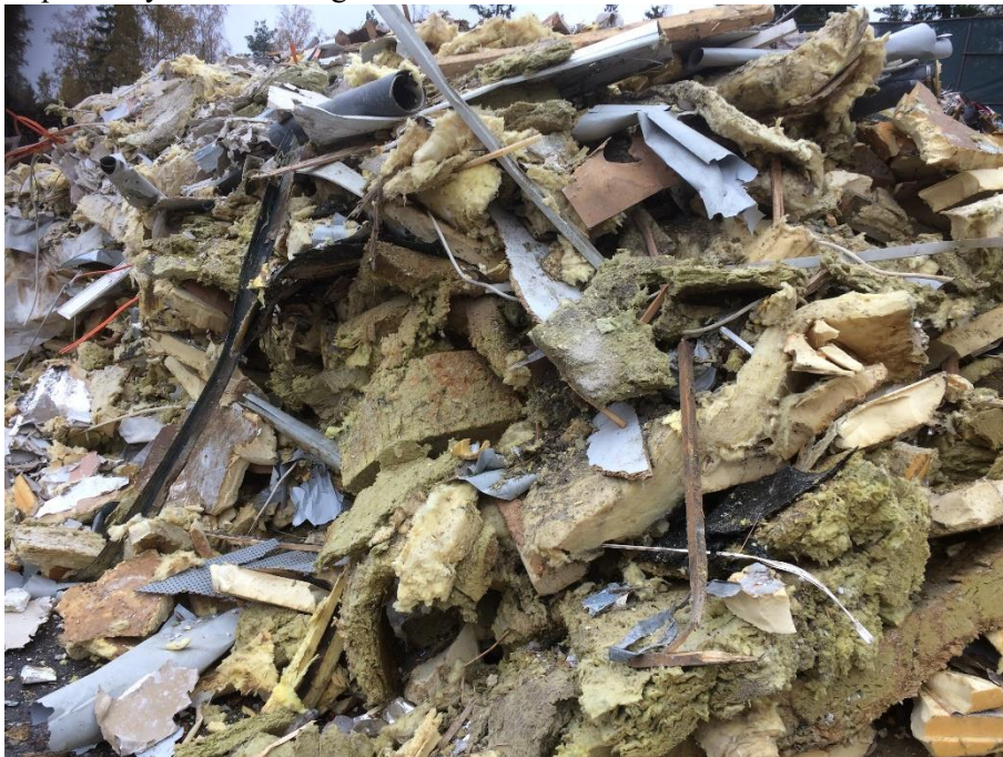
Figure 1. Mineral wool samples were collected manually from demolition and construction sites.
