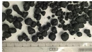
Fig. 73.1 The granulated Petrit-T using Eirich high intensity mixer
