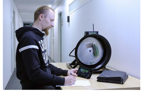
Fig. 3. Wireless sensor node application in a rotating environment enabled with energy transmission.
