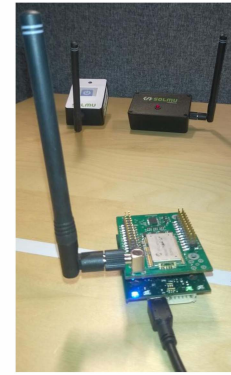
Fig. 4. Powering a printed electronic display and a conventional LED using the LORA radio and energy transmission.
