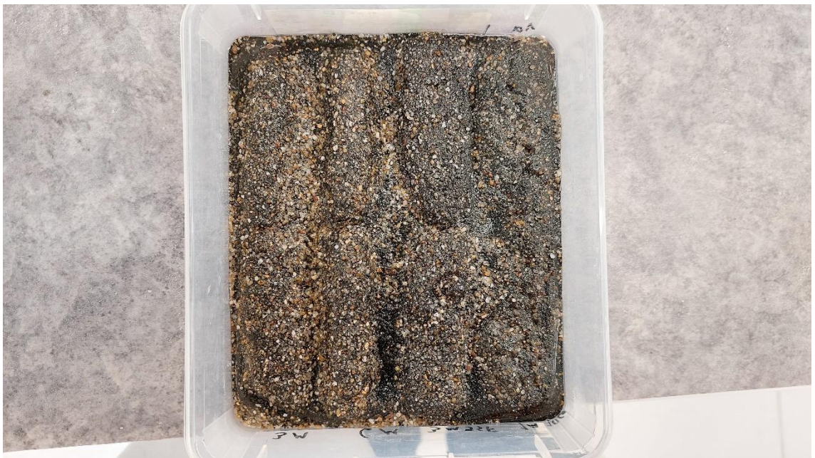
Figure A47. 3M, 6M, 3M-5SF and 1M-10CO mortars after 120 freeze-thaw cycles
