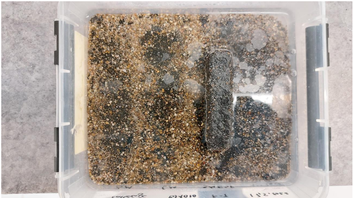
Figure A46. 3M, 6M, 3M-5SF and 1M-10CO mortars after 60 freeze-thaw cycles.
