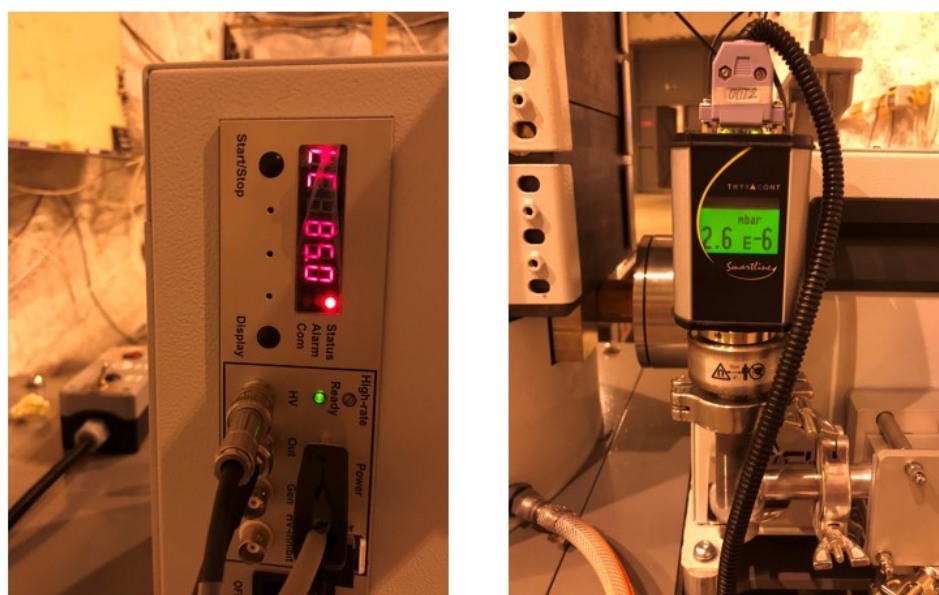
Figure 12. During operation, cryostat temperature should be around 85 K and pressure be in the 10^{-6} mbar range. These should be observed especially during start-up to prevent damage to the spectrometer. The cryocooler and -controller require uninterrupted electrical supply and this should be ensured with UPS units. If there is a break in electricity, the vacuum and operating temperature begin to approach ambient temperatures, and must be restored before continuing measurements. Photo by author.
