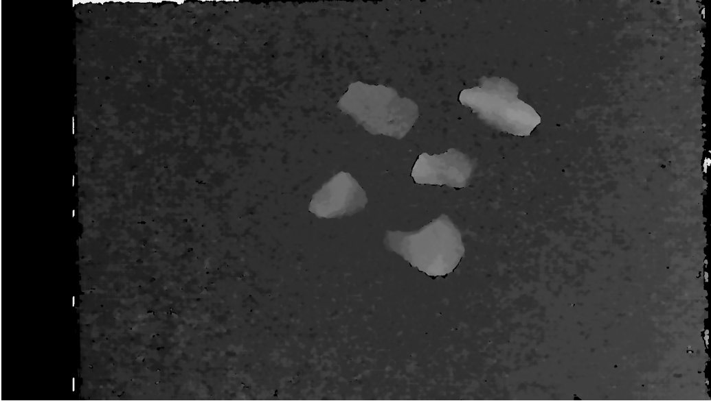
Figure 4.8: Dense disparity image provided by semi-global matching. Image reproduced with permission from Antmicro Ltd.
