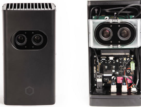
Figure 7.1: Industrial 3-D stereo vision camera system developed by Antmicro Ltd.
