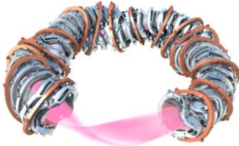
Figure 6. The 50 non-planar superconducting magnet coils (silver) and 20 planar magnet coils (orange) confine the plasma depicted in pink (IPP 2018f).
