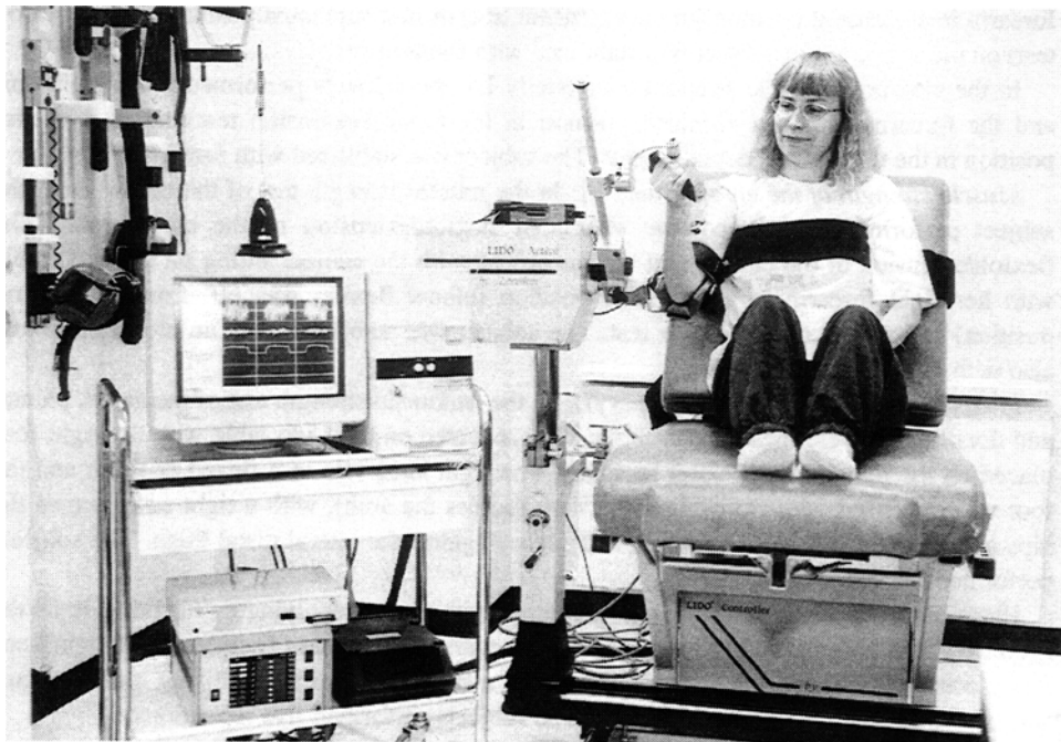
Fig 5. Lido Active Multi-joint and Noraxon Telemyo System, and the measurement of isometric muscle strength and EMG of the hand.
