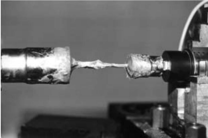
Fig. 2. Torsion testing machine with a bone attached ready to be tested.
