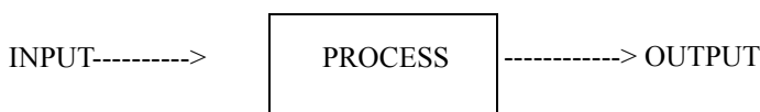
Fig. 1. The principle of the open loop control system (Norman et al. 1995, p. 699).
